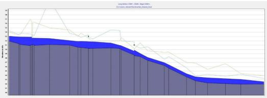
Plate 5 – Longitudinal Profile of Channel 01 with Realigned Channel under Q1000 scenario
